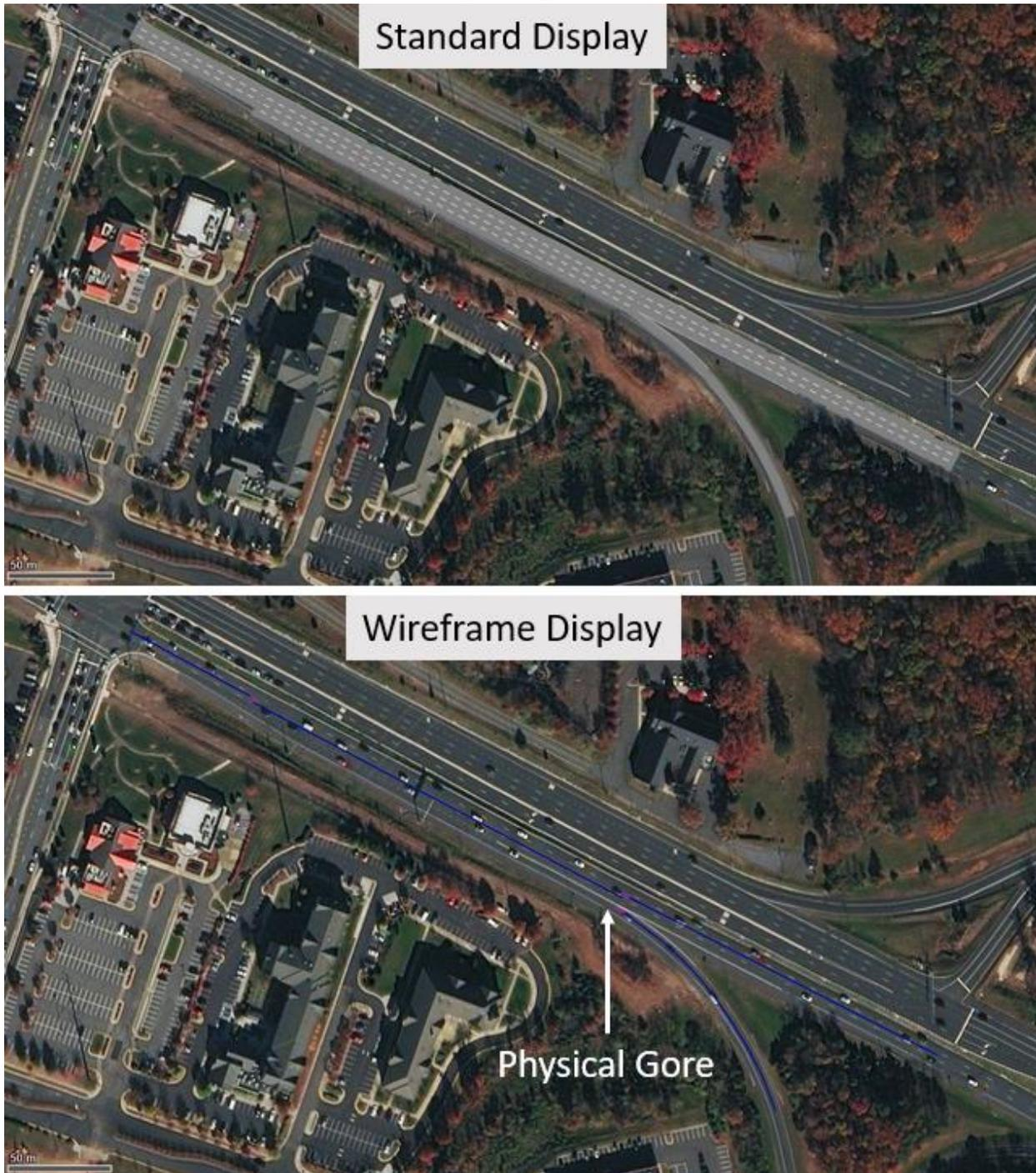
For example, in the merge represented in **Figure 2-10**, the link downstream of the end of the acceleration lane is broken at 700 feet so that the two links together equal approximately 1,500 feet. Results for these two links should be aggregated together to report results for this Merge Segment.
